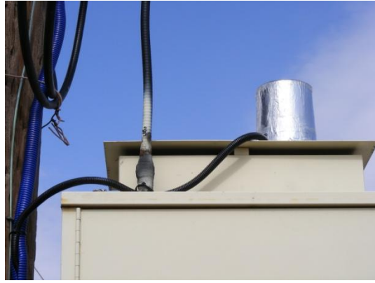
Anemometer is Offset to Clear Pole; Rain Gauge Wrapped in Foil Perched on Cabinet
