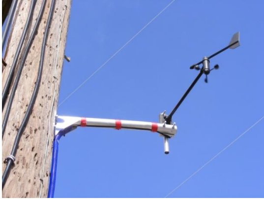
Anemometer is Offset to Clear Pole; Rain Gauge Wrapped in Foil Perched on Cabinet
